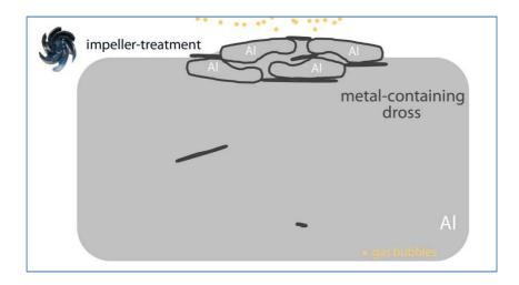
Impeller treatment and fluxing can be combined very well. The process starts with a high rotation speed, there is the formation of a vertex to distribute the flux and generate a reaction with the impurities and the melt.
