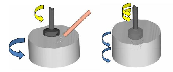
For the actual cleaning process the rotor rotates with a lower rotation speed. It rotates in the opposite direction as the melt. So the relative motion between melt and rotor is very high, the resulting bubbles are very small, and no vertex is created. Once the melt rotates in the same direction as the rotor, the rotor changes its direction (this happens 3 or 4 times per cleaning process).
