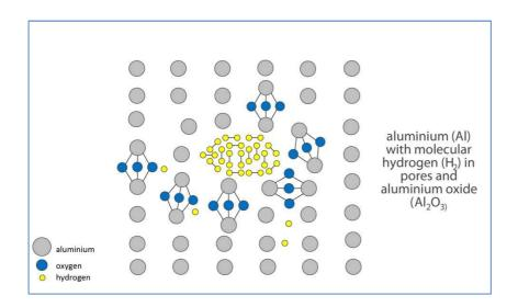
During a casting process, the aluminium is surrounded by an oxide skin; some of the oxides will get into the melt, too. The oxides can have the shape of skins with a very high length to width ratio; some of the skins include or surround some aluminium drops, too.
