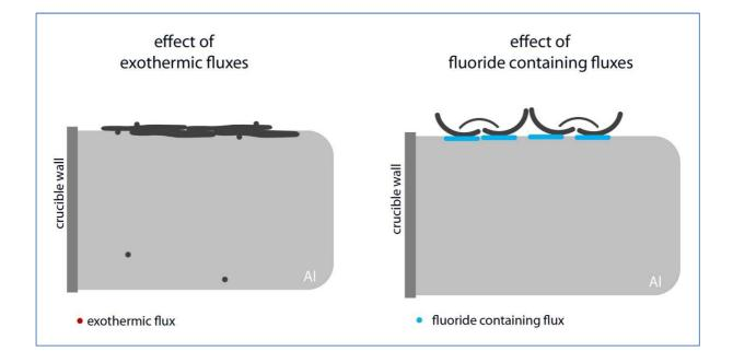
Both types of fluxes are creating a low metal dross, but the exothermic ones do not remove the oxides from the melt, they even create new ones, and so increase the building up of corundum at the crucible walls.
