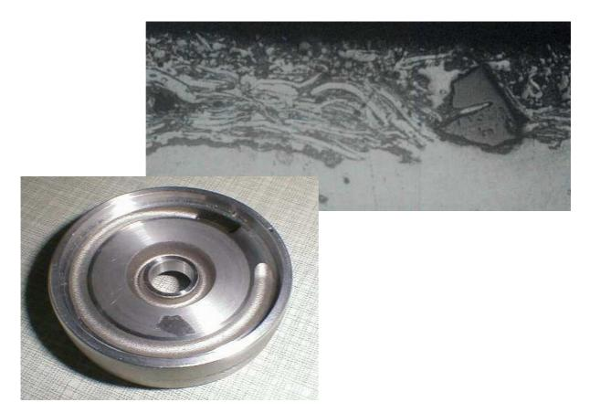
This is a high pressure die casting with a very hard inclusion. During the machining process the tooling was destroyed by this. A metallographic examination could show some corundum and agglomerates of oxides in this area.
