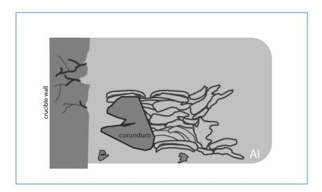
In the melt you can find some oxides, there are micro cracks in the wall. There is some sticking of the oxides at the wall, some oxides even diffuse into the micro cracks. Depending on time and temperature, some crystallization of the oxides to corundum takes place, at which the micro cracks are opened more. If the crystallization continues, some pieces of corundum can get into the melt, too.
