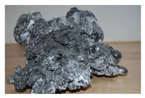
Without the use of a flux the metal content is very high, normally between 80 and 95 %. If a flux is used, the dross is fluffier, and the metal content between 20 and 35%:
