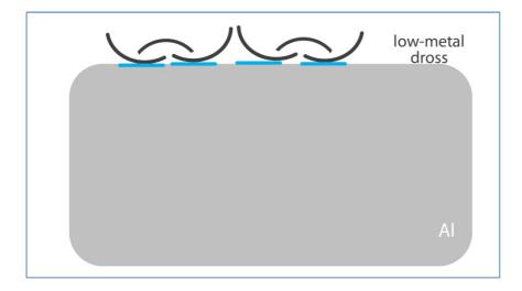
The cleaning process with fluxes can be combined very well with an impeller treatment. So an optimal degassing and removing of oxides combined with a low metal dross in guaranteed.
