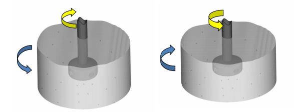
For this highly effective impeller process no ceramic baffle is needed.
