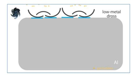
Without a flux, the impeller treatment is not so effective in removing all oxides, and the dross will be metal rich in the end.
