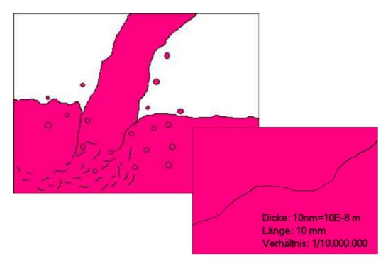
The release of hydrogen, that means the building up of bubbles, takes place at interior defects in the melt and lattice of aluminium, oxides act as nuclei for the bubbles:
