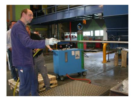
Best the furnace cleaner is sprayed on the walls.
