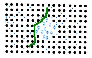
There is a critical radius for bubbles: Bubbles with a radius higher as 0,32 nm will grow, their surface tension is low, smaller ones can collapse, having a high surface tension and only a low inner pressure.
