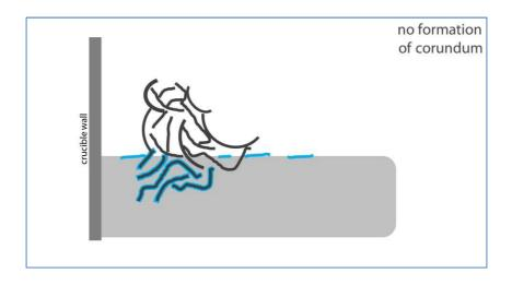
The oxides are covered by the flux, as shown before. There is only a loose connection of them to the crucible wall, and the most important thing is, that there is NO crystallization to corundum. The loose adherences to the crucible wall can be removed very easily during taking away of the dross.
